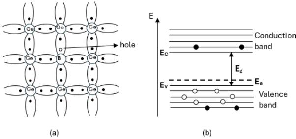
Figure 1.4: (a) p-type semiconductor (b) Energy band diagram of p-type semiconductor at  $T > 0K$
