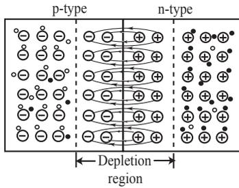
Figure 1.9: Space charge formed at the junction
