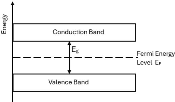
Figure 1.2: Fermi level in intrinsic semiconductor
