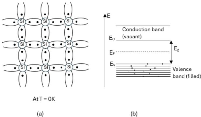
Figure 1.1: (a) Silicon crystal at 0K (b) Corresponding energy band diagram
