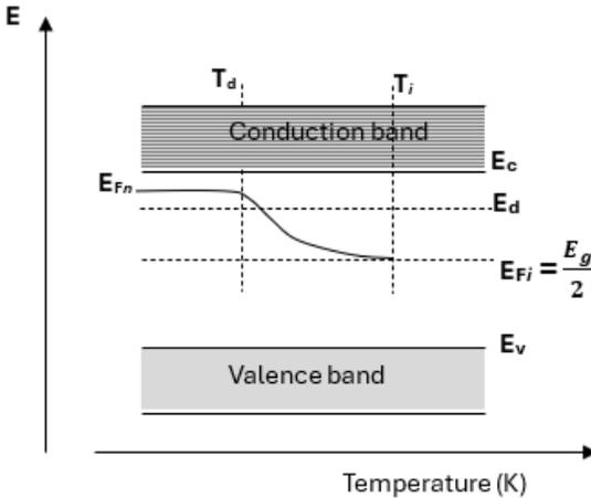
Figure 1.5: Qualitative dependence of Fermi level on temperature in an n-type semiconductor
