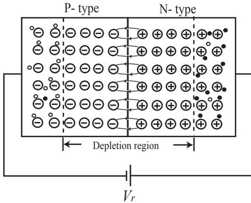
Figure 1.12: Reverse biased p-n junction
