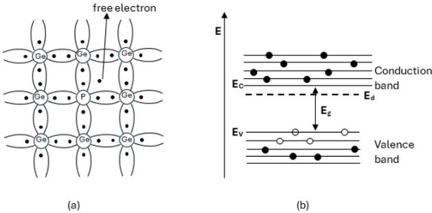
Figure 1.3: (a) n-type semiconductor (b) Energy band diagram of n-type semiconductor at  $T > 0K$
