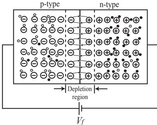
Figure 1.11: Forward biased p-n junction
