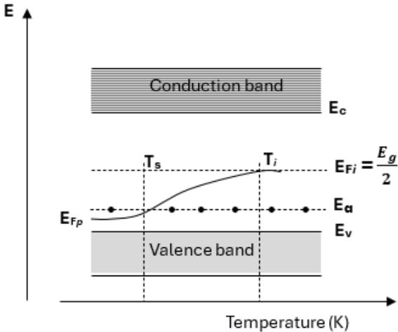
Figure 1.6: Qualitative dependence of Fermi level on temperature in an p-type semiconductor
