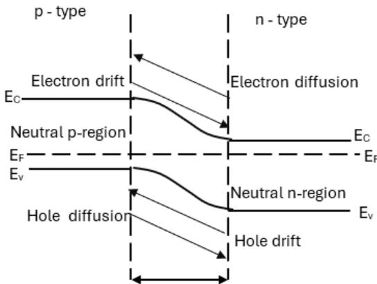
Figure 1.10: Energy band diagram of pn junction
