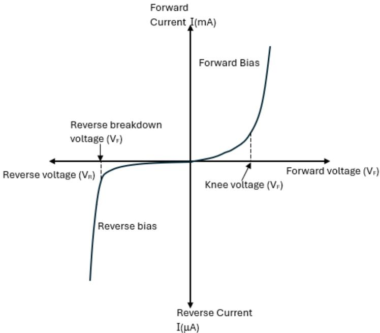
Figure 1.13: V-I characteristics of diode
