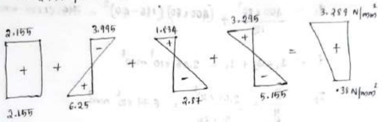
8) An asymm. I S/c beam is used to support an imposed load of 4 kN/m over a span of 12m. The S/c details are top flange 400mm wide & 80mm thick, bottom flange 150mm wide and 80mm thick, thickness of web is 100mm. Overall depth of beam is 500mm. At the centre of span effectively prestress force is 150 kN is located at 80mm from the soffit of beam. Estimate stress at centre of the span of beam for following conditions:
