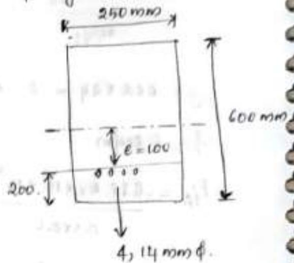
$$f_{\text{bottom}} = \frac{P}{A} + \frac{Pe}{Z} - \frac{M}{Z}$$
