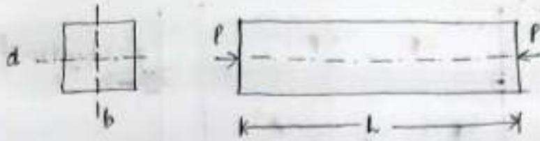
$$\text{direct stress} = +P/A \quad (P = \text{compressive force})$$
