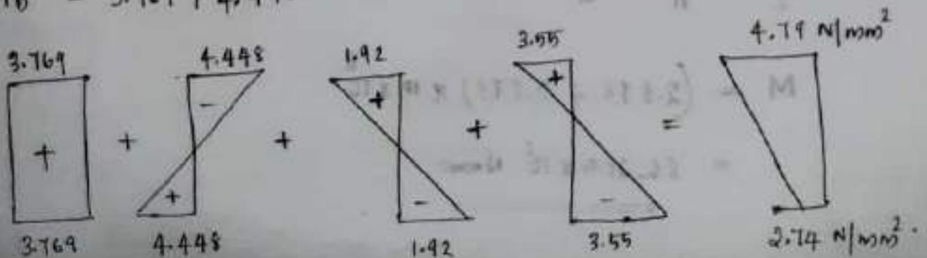
5) A rectangular concrete beam <sup>(wide)</sup> 250 mm x <sup>(deep)</sup> 600 mm is prestressed by means of 4 nos. of 14 mm  $\phi$  wires located 200 mm from soffit of beam. If the effective stress in wire is 700 N/mm<sup>2</sup>. What is max bending moment that can be applied to it without causing tension at the soffit of beam.
