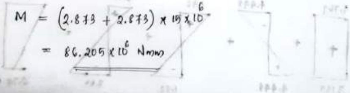
6) A prestressed concrete beam of size  $200 \text{ mm} \times 300 \text{ mm}$  is used over an effective span of  $6 \text{ m}$  to support an imposed load of  $4 \text{ kN/m}$ . Density of concrete =  $24 \text{ kN/m}^3$ . At the centre of span of the size of beam find magnitude of (a) the concentric prestressing force necessary for zero fibre stress at soffit when beam is fully loaded
