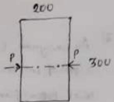
$$(b) f_{bottom} = \frac{P}{A} + \frac{Pe}{Z} - \frac{mg}{Z} - \frac{m_j}{Z}$$
