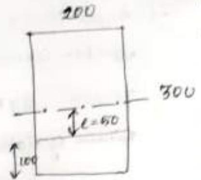
7) An unsym. I/c beam is used to support an imposed load of 2 kN/m over a span of 8m. The sectional details are top flange 300 mm wide & 60 mm thick. Bottom flange 100 mm wide and 60 mm thick. thickness of web is 80 mm. Overall depth of beam is 400 mm. At the centre of span, the effective prestressing force 100 kN is located at 50 mm from the soffit of the beam. Estimate stress at centre of span of beam for following conditions-
