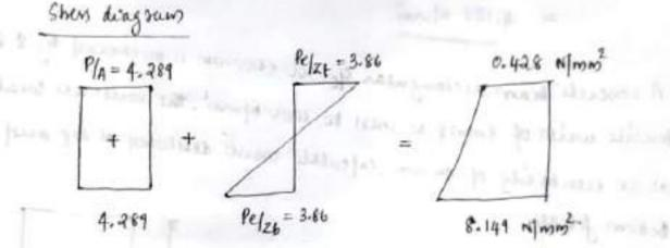
A vectorgular concrete beam C/s of 30 cm deep \$ 20 cm while is prestress by 15 where of through tocalied at a distance of 6.5 cm from bottom of beam and 3 wikes of through is wealth at a distance of 2.5 cm from top. Assum prestress in steel is \$40 N/mm<sup>2</sup>. cafeculate shen@ extreme fibre of midspass she when beam is supporting it own weight over a span of 6m if upl of 6 km/m is imposed. cafeculate max shess in concrete. Assume density of converte - 24 km/m<sup>3</sup>.
