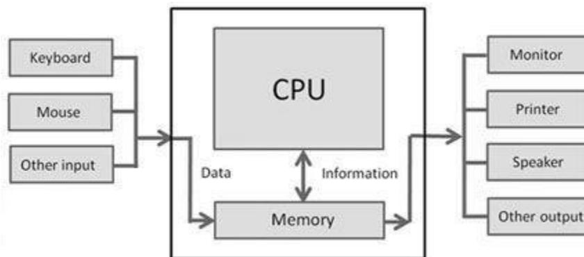
The basic components of a modern digital computer are: Input Device, Output Device, Central Processor Unit (CPU), mass storage device and memory.
