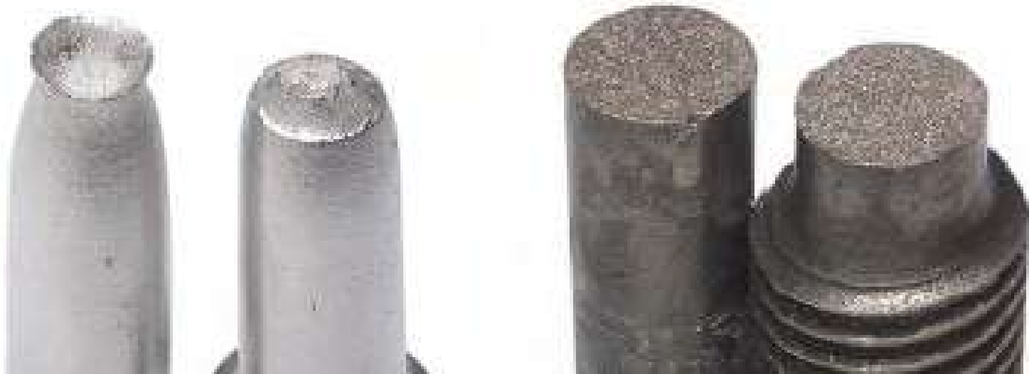
(a) Cup-and-cone fracture in aluminum. (b) Brittle fracture in a mild steel.
